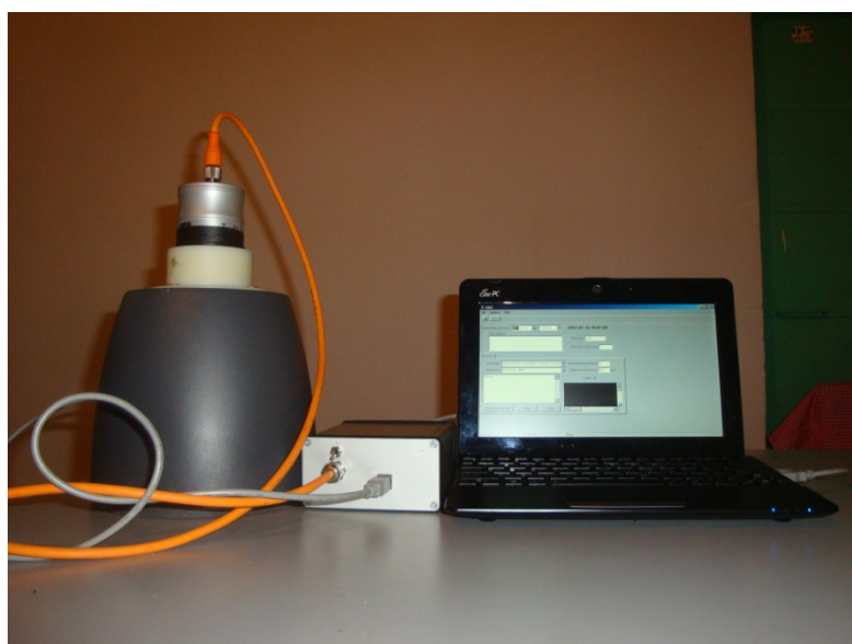
Fig. 1 Soil respirometer: chamber with the Vaisala GMP 343 CO 2 sensor, interface, and computer.
